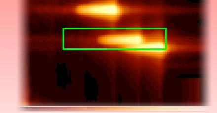
more sources are inside the same window; fitting the data with template spectra or Gaia spectra will disentangle the spectra while also computing the background
