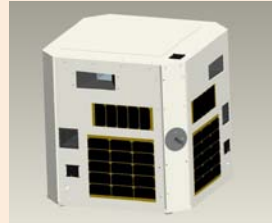
Figure 1: The external appearance of NJ. It is about 50 cm cubic in size and weighs about 30 kg.
