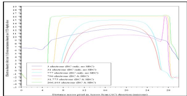
Figure 3: Silvaco pixel model-simulated AC electron density profiles through different sized charge packets. The AC cut is the same as in Fig. 1 i.e. there is half a ABD at 0-1  $\mu\text{m}$  and another half a ABD at 29-30  $\mu\text{m}$ . The SBC (at around 27-28  $\mu\text{m}$ ) causes the bimodal distribution at low signal size (when it is present in the simulation) and the BC runs from 4.5 to 28.
