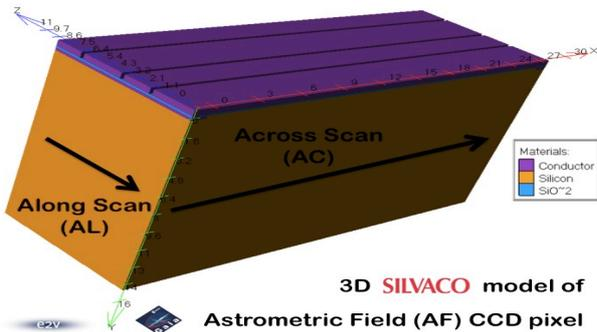
Figure 1: 3D Silvaco model of a single AF CCD pixel. In the AL direction, the model has 4 electrodes that make up 1 pixel. In the AC direction, the model runs from half way through one Anti-Blooming Drain (ABD, seen above as a conductor region beneath the oxide) to half way through the next ABD, delineating 1 CCD column.
