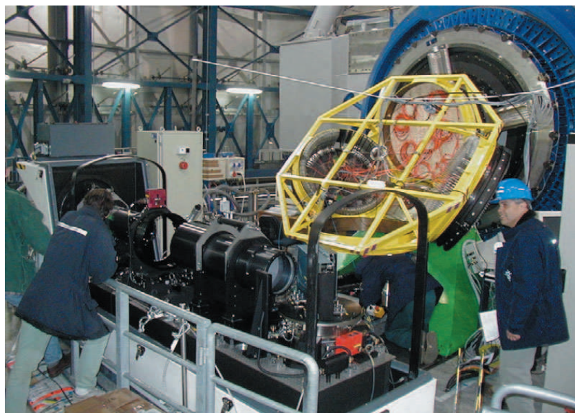
Figure 1: The fibre positioner and GIRAFFE as seen during the GIRAFFE integration on the Nasmyth platform. The positioner is looking towards the Nasmyth Focus, where the corrector is placed (only the corrector support is visible). GIRAFFE is open, and all the optomechanics components are visible. The picture was taken when the OzPoz enclosure had not yet been installed.
